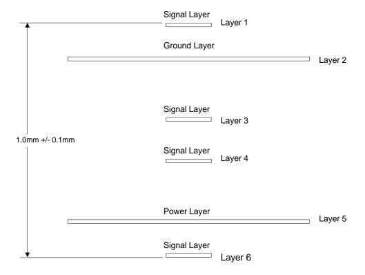
Figure 10: Example 6-layer PCB Stackup
