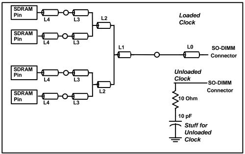
Note: Either the L2 or the L3 trace segment may contain one additional via which is not shown in the diagram.
