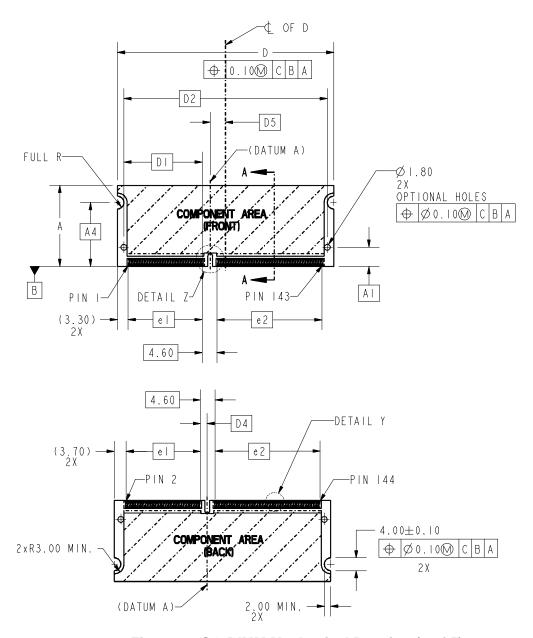
Figure 3: SO-DIMM Mechanical Drawing (1 of 5)
