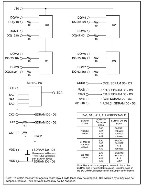
Figure 8: 64-bit non-ECC SO-DIMM Block Diagram (1 Row, x16 SDRAMs)
