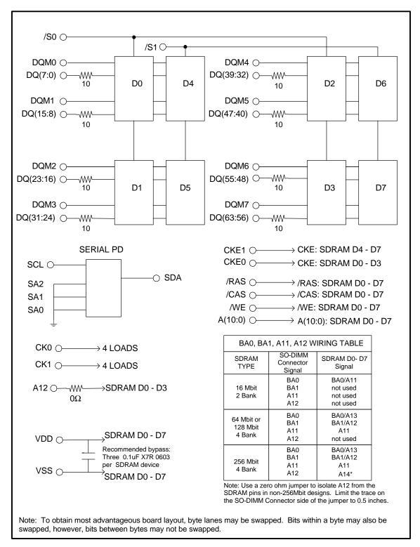
Figure 9: 64-bit non-ECC SO-DIMM Block Diagram (2 Rows, x16 SDRAMs)
