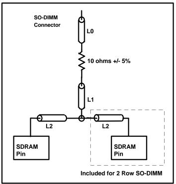
Figure 13: Signal routing topologies for Data
