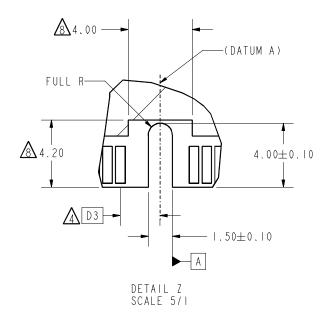
Figure 5: SO-DIMM Mechanical Drawing (3 of 5)
